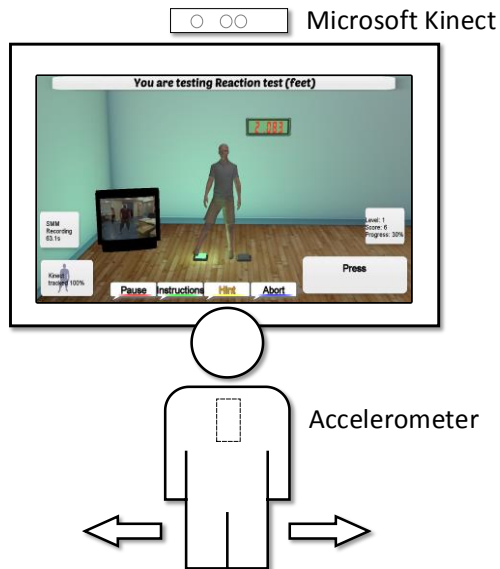
Fig. 1. Schematic representation of the sensor-based Exergame Choice Stepping Reaction Test. Participants were asked to step laterally as quickly as possible after a light stimulus, indicated by the Exergame, appeared on the TV screen.
